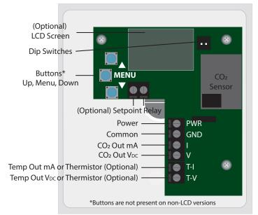
4. Set DIP switch positions to accomodate your application. DIP switch 2 only applies to units with transmitter temperature output selected.
